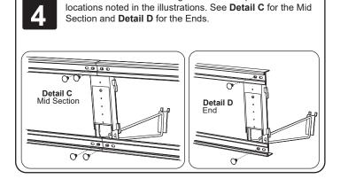
Secure the Extrusions using Xmas Tree Clips. Use the hole
